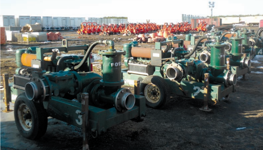
Foss six-inch pumps are ready to be deployed from Lakehurst (N.J.) Naval Air Station.
