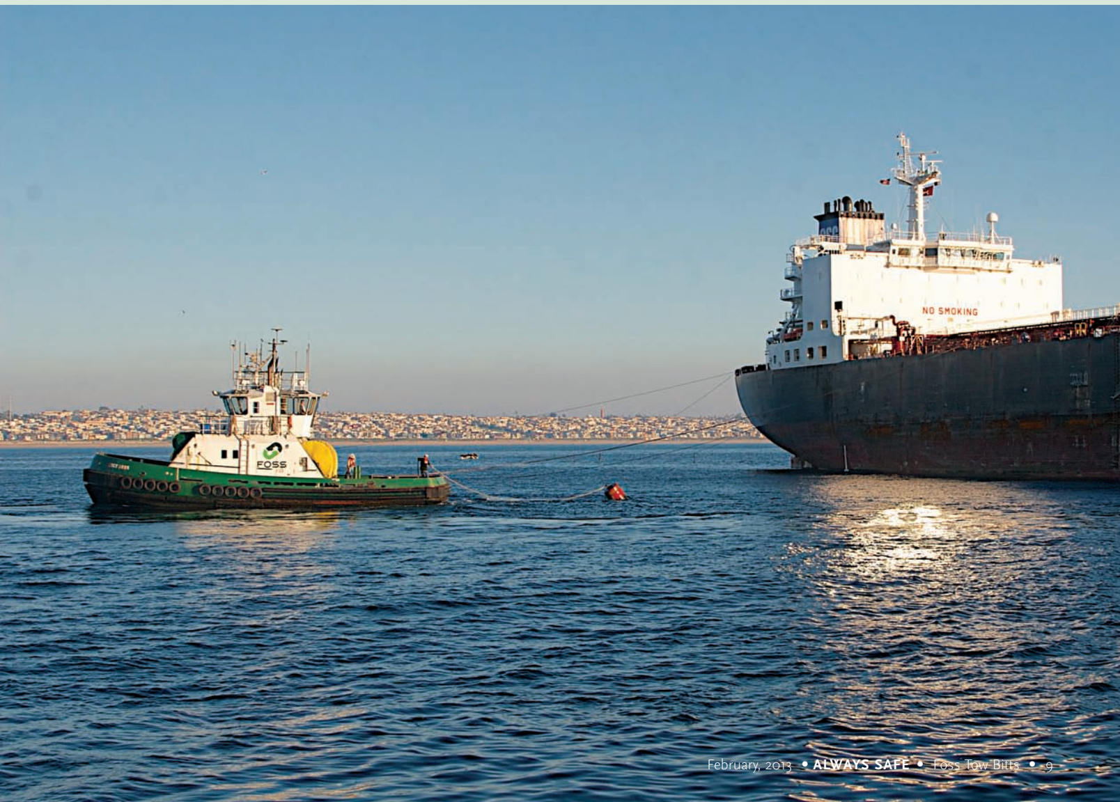
The Lucy Foss , below, tows a buoy attached to a crude oil line away from a tanker at the moorings.
